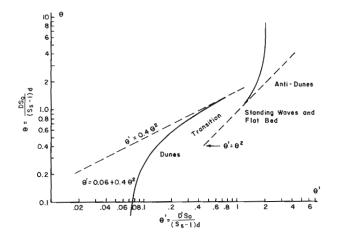
Figure 4-4.—Relationship between dimensionless forms of bed shear ( $\theta$  and  $\theta'$ ). From Engelund and Hansen (1967) and American Society of Civil Engineers (1975, p. 135).
