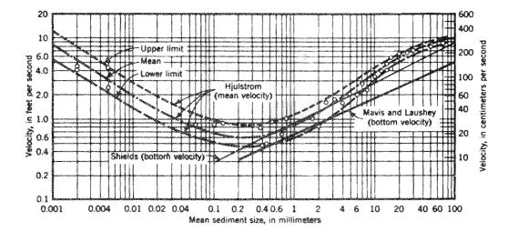
Figure 4-1b.—Critical water velocity for quartz sediment as a function of mean grain size. From American Society of Civil Engineers (1975, p. 102).
