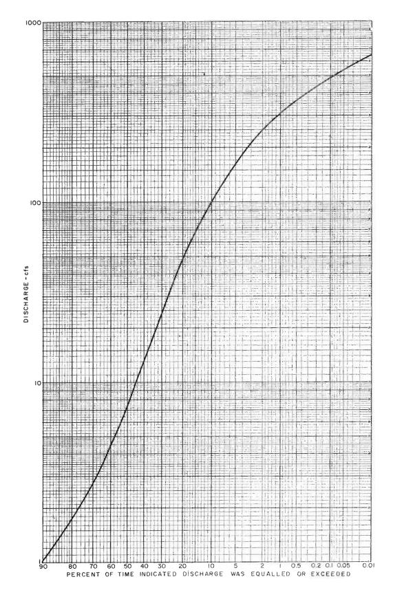
Figure 4-14.-Flow-duration curve, Cottonwood Creek, any State.
