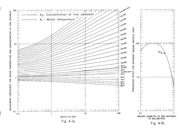
Figure 4-7.—Approximate correction factors for the effect of water temperature and concentration of fine sediment (4-7a) and sediment size (4-7b) on the relationship of discharge of sands to mean velocity. From Colby (1964) and American Society of Civil Engineers (1975, p. 205).
