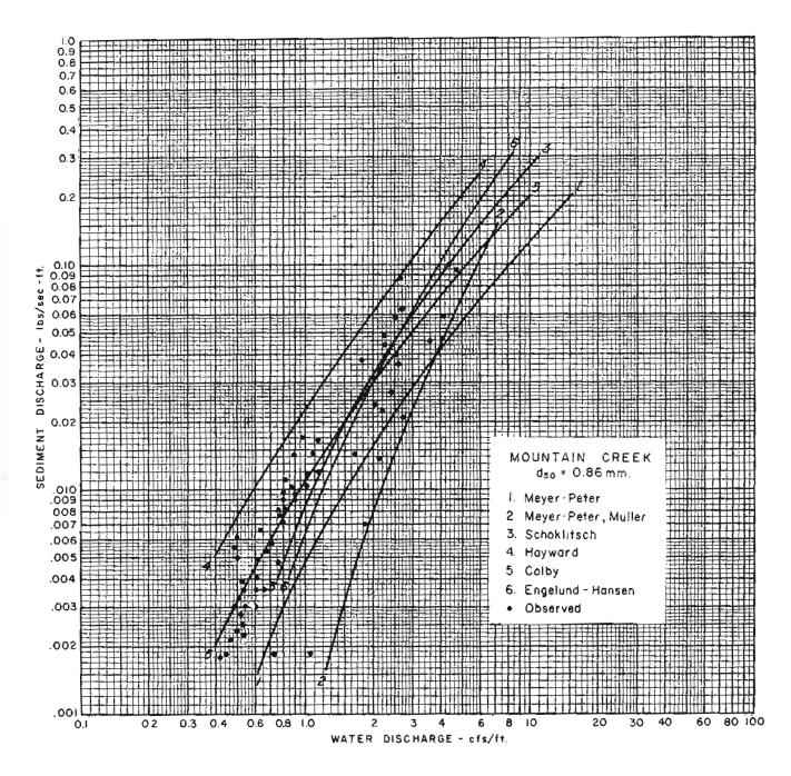
Figure 4-9.—Sediment rating curves for Mountaín Creek near Greenville, S.C., according to several formulas compared with measurements. Adapted from Vanoni, Brooks, and Kennedy (1961, p. 7-8).
