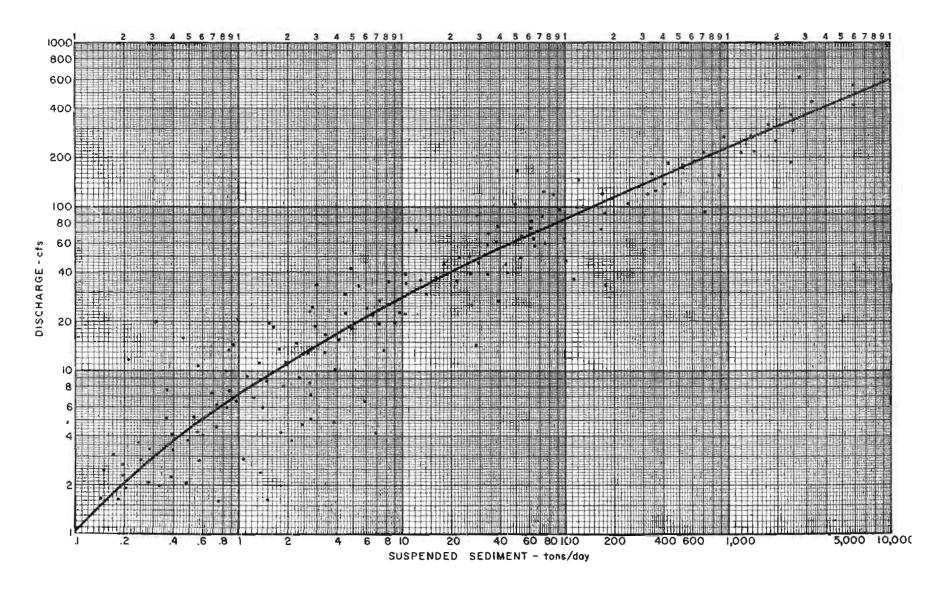
Figure 4-13.-Sediment rating curve, Cottonwood Creek, any State.
