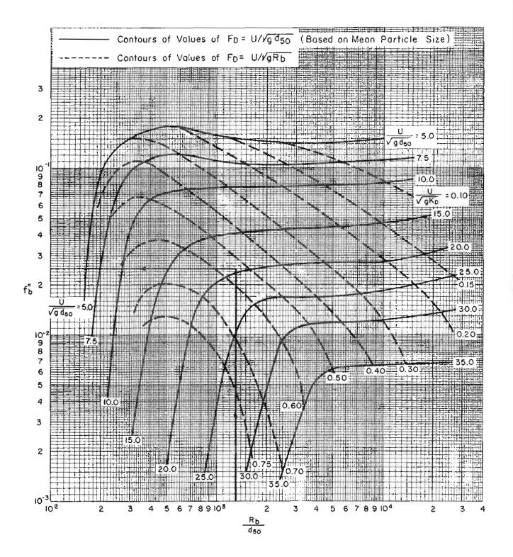
Figure 4-15.--Form-drag friction factor in sand-bed channels,  $f_b''$ , as a function of  $R_b/d_{so}$  and  $F_D = U/\sqrt{gd_{so}}$ . From Alam and Kennedy (1969), American Society of Civil Engineers (1975, p. 142).
