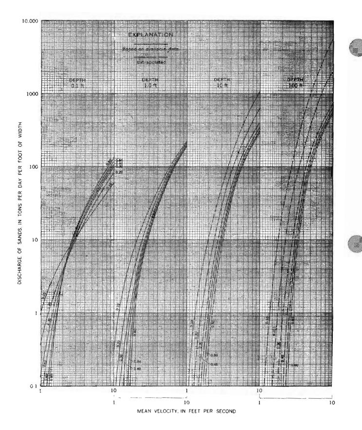
Figure 4-6.—Relationship of discharge of sands to mean velocity for six median sizes of bed sand, four depths of flow, and a water temperature of 60° F. From Colby (1964) and American Society of Civil Engineers (1975, p. 204).
