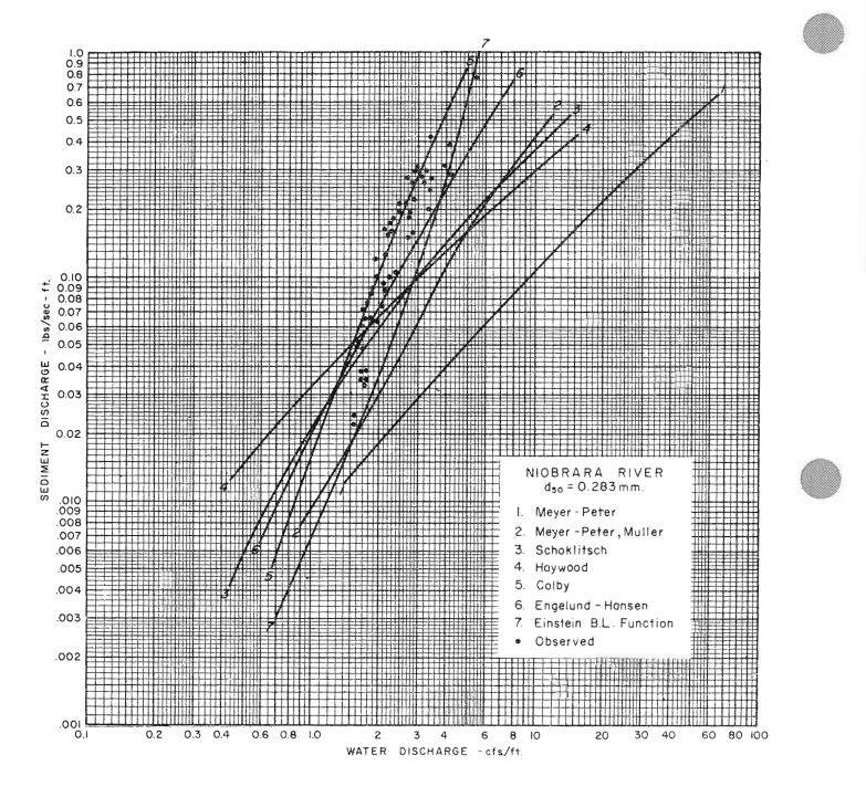
Figure 4-10.—Sediment rating curves for Niobrara River near Cody, Nebr., according to several formulas compared with measurements. Adapted from Vanoni, Brooks, and Kennedy (1961); American Society of Civil Engineers (1975, p. 221).
