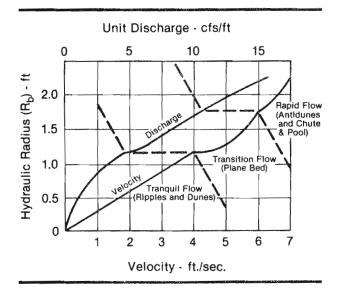
Figure 4–17.—Depth-discharge relationships obtained by Alam-Kennedy technique.
