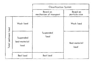
Figure 4-2.—Sediment load classification. Adapted from Cooper and Peterson (1970, p. 1,881).
