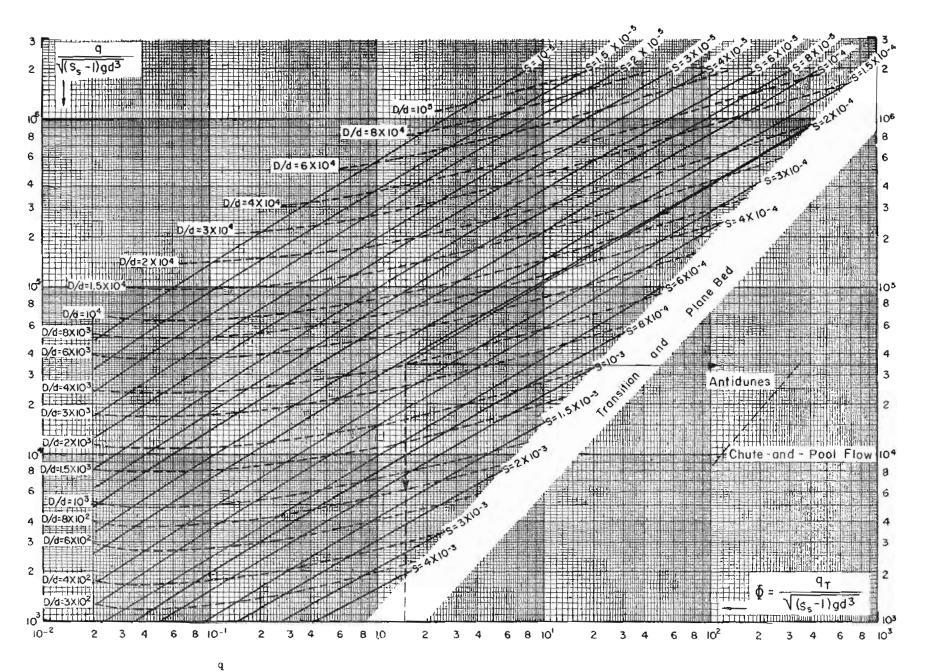
Figure 4-5.—Graphical solution to  $\sqrt{(S_{a} - 1)gd^{3}}$  and  $\phi$  in the Engelund-Hansen procedure. Adapted from Engelund and Hansen (1967) and American Society of Civil Engineers (1975, p. 209).
