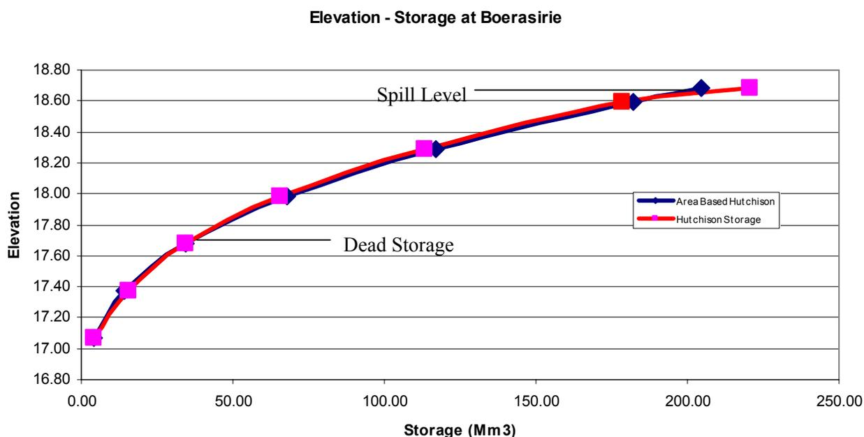
**Figure 4.2** Elevation – storage curve for Boerasirie Conservancy (Hutchinson, 1951)
