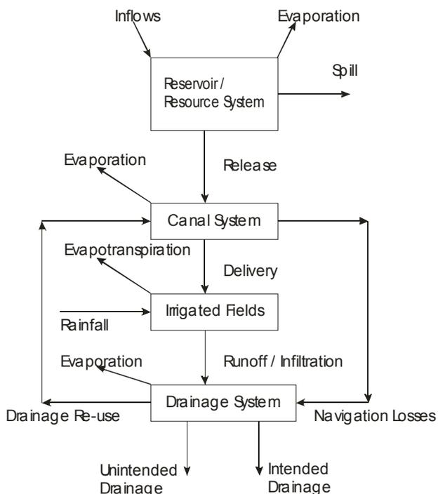
**Figure 4.1** Schematic of the drainage and irrigation system
